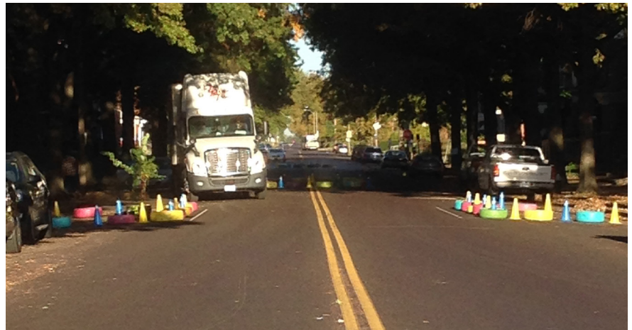
TEMPORARY BUMP-OUTS CREATING NARROW LANES ON DEMONSTRATION DAY
